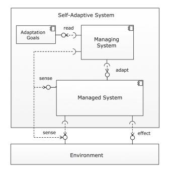
Figure 3.1: Conceptual model of self-adaptive system [1]
